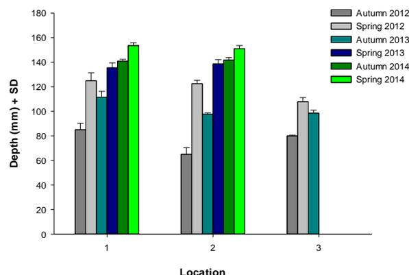
Figure 6. Average plate depth at each location over the 6 surveys, i.e. cumulative deposition. The difference between autumn and spring 2012 pre-construction surveys equates to initial plate settlement.
